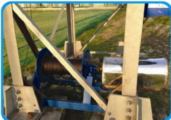
The pulley, cable, and net hoist system
